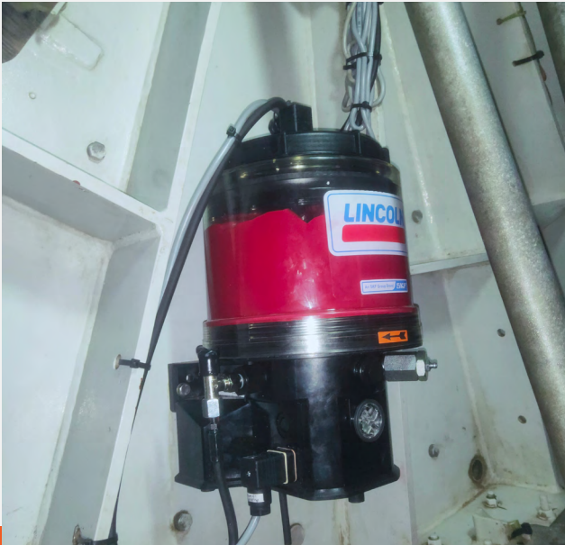
Installed CLS system in Spinner Area of WTG
